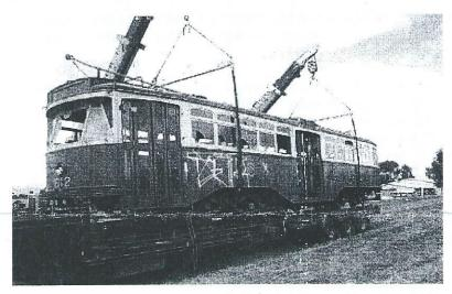
"Yapper, Yapper, Doo". With the cranes in position Y1 612 is about to be lifted from the road transport vehicle onto rails at Bylands. The acquisition of this vehicle fulfils a long time dream to have one of these rare vehicles in our collection. Unfortunately the vehicle had suffered some vandalism prior to its departure from Melbourne, some of the broken windows and graffiti highly visible.
